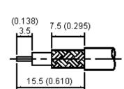
**Stripping Dimension** Dimensions : Millimetres (Inches)
