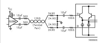
FIGURE 13. Twisted Pair Equalization
