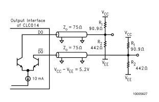
FIGURE 7. Alternative Load Terminated Output Interface
