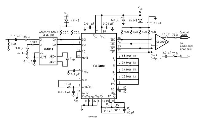
FIGURE 11. Typical Repeater Design
