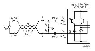
**FIGURE 4. Twisted Pair Input Interface**
