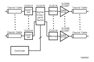
FIGURE 12. Video Routing Block Diagram
