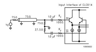
FIGURE 3. Single-Ended 75 $\Omega$  Cable Input Interface
