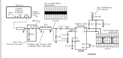
FIGURE 15. Typical Measurement Setup
