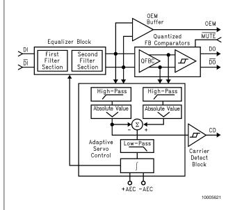
FIGURE 2. CLC014 Block Diagram
