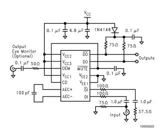
FIGURE 1. CLC014 Equalizer Application Circuit
