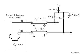
FIGURE 5. Differential Load Terminated Output Interface
