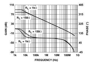
FIGURE 8. OPEN LOOP GAIN AND PHASE vs FREQUENCY
