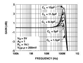
FIGURE 5. SMALL SIGNAL FREQUENCY RESPONSE FOR VARIOUS  $\mathbf{C}_{L}$
