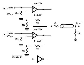
FIGURE 29. TWO TO ONE MULTIPLEXER
