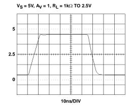
FIGURE 19. LARGE SIGNAL TRANSIENT RESPONSE
