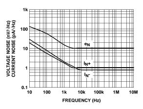
FIGURE 18. VOLTAGE AND CURRENT NOISE vs FREQUENCY
