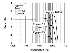
FIGURE 1. FREQUENCY RESPONSE FOR VARIOUS OUTPUT **VOLTAGE LEVELS**
