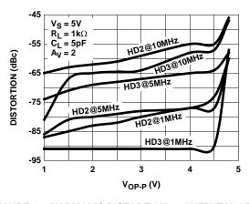
FIGURE 14. HARMONIC DISTORTION vs OUTPUT VOLTAGE
