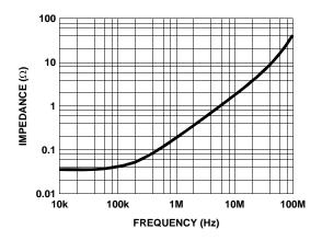
FIGURE 11. OUTPUT IMPEDANCE vs FREQUENCY
