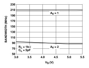
FIGURE 10. SMALL SIGNAL BANDWIDTH vs SUPPLY VOLTAGE
