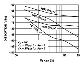
FIGURE 17. HARMONIC DISTORTION vs LOAD RESISTANCE
