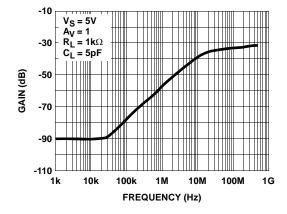
FIGURE 15. DISABLED OUTPUT ISOLATION FREQUENCY **RESPONSE**
