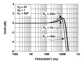
FIGURE 2. SMALL SIGNAL FREQUENCY RESPONSE FOR **VARIOUS RLOAD**
