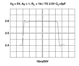
FIGURE 21. SMALL SIGNAL TRANSIENT RESPONSE
