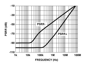
FIGURE 13. POWER SUPPLY REJECTION RATIO vs **FREQUENCY**
