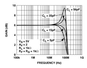
FIGURE 6. SMALL SIGNAL FREQUENCY RESPONSE FOR VARIOUS  $\mathbf{C}_{L}$
