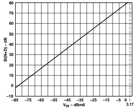
Figure 5c. S/(N+D) vs. V_{IN} (ADC @ 5 V) over Voiceband Bandwidth (300 Hz – 3.4 kHz)
