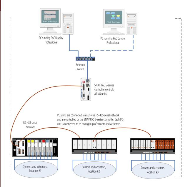
This diagram shows a SNAP PAC S-series controller connected to multiple Opto 22 serial-based I/O units over an RS-485 serial network. The controller is also connected to a larger, separate enterprise Ethernet network to provide process data to a PC running Opto 22's PAC Display HMI software.
