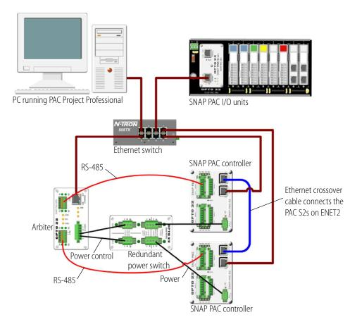
In this diagram, two S-series controllers are operating redundantly. One is the active controller, while the other acts as a backup, ready to take over should the first one fail.
