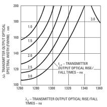
HFBR-5905 TRANSMITTER TEST RESULTS OF  $\lambda_{c}, \Delta\lambda$  AND  $t_{cr}$  ARE CORRELATED AND COMPLY WITH THE ALLOWED SPECTRAL WIDTH AS A FUNCTION OF CENTER WAVELENGTH FOR VARIOUS RISE AND FALL TIMES.
