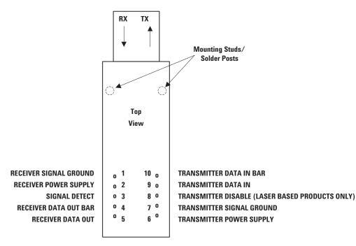
Figure 3. Pin Out Diagram.
