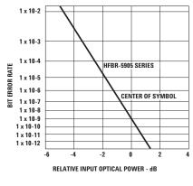
CONDITIONS: 1. 125 MBd 2. PRBS 2<sup>7</sup>-1 3. CENTER OF SYMBOL SAMPLING 4.  $T_A = +25C$ 5.  $V_{cc} = 3.3 V dc$ 6. INPUT OPTICAL RISE/FALL TIMES = 1.0/2.1 ns.
