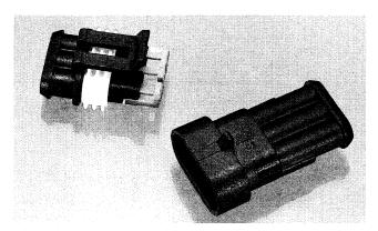
Secondary locks are factory installed on all connector housings. Plug connectors include a factory installed interface seal. Connector housings and secondary locks are made from glass filled nylon.
