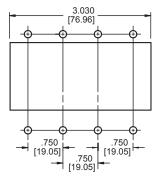
Panel Mounting Detail: Tolerance ±.005 [.13] Unless noted.
