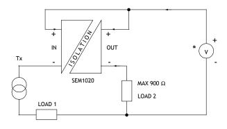
Used to increase the limited drive capability of a intriniscally safe (4 to 20) mA loop
