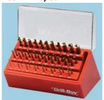
Ground flute high speed steel Jobber drills. Ideal for general workshop or maintenance use. Supplied in polycarbonate storeage case incorporating a drill gauge to size drills. 1mm - 13mm in 0.5mm increments. Tapping drill sizes 3.3mm, 4.2mm, 6.8mm and 10.2mm.
