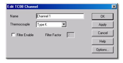
9. From the Thermocouple drop-down list, select the type of thermocouple you are using and click the OK button.
