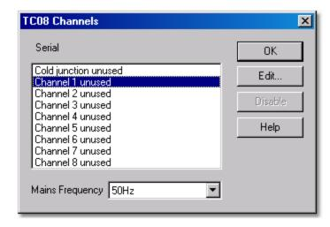
8. In the TC-08 Channels window, double-clickon Channel 1 unused The Edit TC-08 Channel dialog box appears
