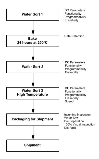
Figure 1. AMD KGD Product Test Flow
