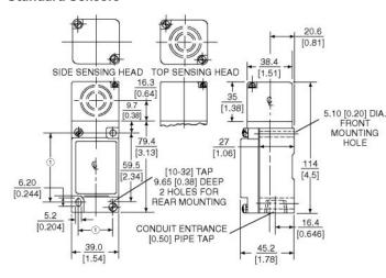
$^{\scriptsize \textcircled{1}}$  Can accommodate both U.S., 29.4 [1.16] x 59.5 [2.34] and DIN, 30 [1.18] x 60 [2.36], mounting dimensions.
