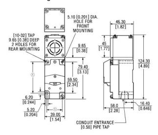
$^{\circledR}$  Can accommodate both U.S., 29.4 [1.16] x 59.5 [2.34] and DIN, 30 [1.18] x 60 [2.36], mounting dimensions.
