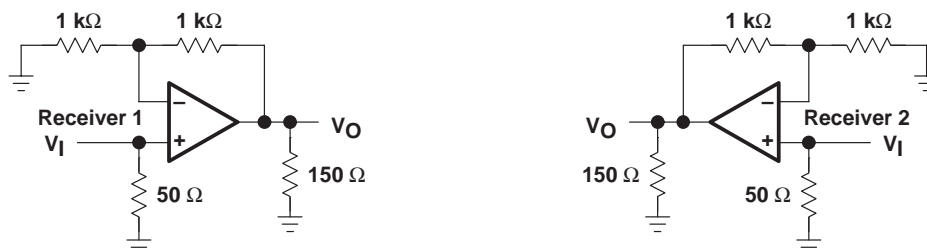
Figure 2. Receiver Input-to-Output Crosstalk Test Circuit
