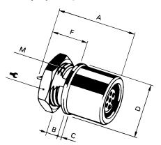
The larger portion of the «DB» is on the outside and occupies less space inside the equipment than the «D».
