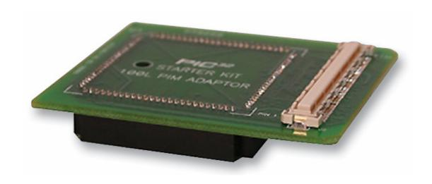
This adapter enables PIC32 Starter Boards to connect to the Plug-In Module on Explorer 16. Users can utilize the functionality on the Explorer 16 or connect PICtail Plus daughter cards for application-specific development.
