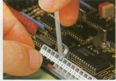
For factory wiring of PCB terminal strips these operating tools are extremely useful to reduce wiring time.
