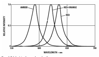
Figure 1. Relative intensity vs. peak wavelength
