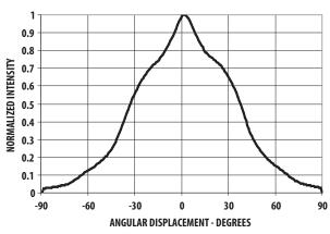
Figure 5. Representative Radiation pattern for 30°x70° Lamp -Major Axis
