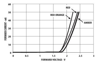
Figure 2. Forward current vs. forward voltage
