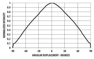
Figure 7. Representative Radiation pattern for 40°x100° Lamp - Major Axis
