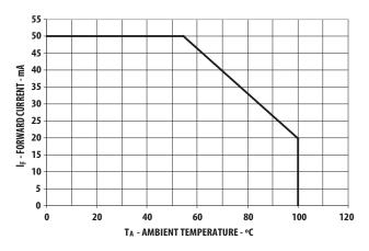
Figure 4. Maximum forward current vs. ambient temperature
