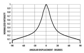
Figure 8. Representative Radiation pattern 40°x100° Lamp – Minor Axis
