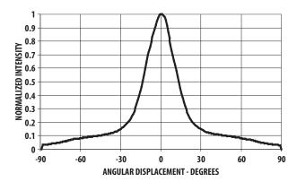
Figure 6. Representative Radiation pattern 30°x70° Lamp -Minor Axis
