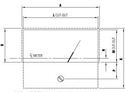
6.00mm/0.24" hole required when optional front zero is specified
