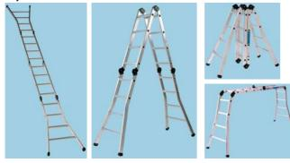
Multi-purpose ladder system, constructed from heavy duty aluminium with splayed legs for extra rigidity. Suitable for use as a straight ladder, step ladder or workbench. Positive locking rust-proof hinges and grooved rungs for safety Conforms to EN131.
