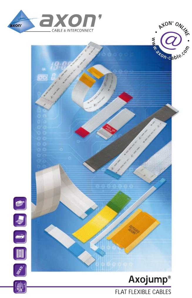
AXOJUMP® Flat Flexible Cables consist of flat tin plated copper conductors insulated between Polyester based tapes. Depending on the type of interconnection used, reinforcement tapes can be added to the cable ends to allow for connector compatibility.
