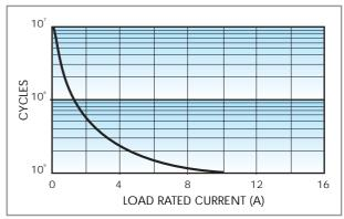
Electrical life vs AC1 load. Type 48.62 (10 A).
