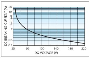
Breaking capacity for DC1 load.
