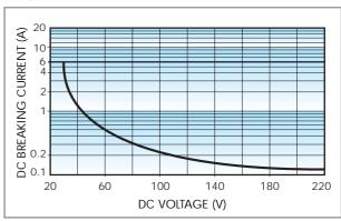
Breaking capacity in DC1 load.
