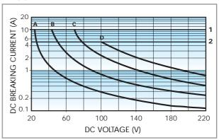
Breaking capacity for DC1 load.
