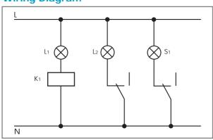
Typical application with current sensing relays.
