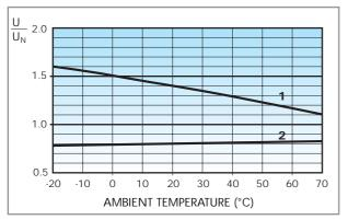
Operating range (AC version) vs ambient temperature.
