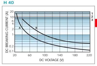
Breaking capacity for DC1 load.
