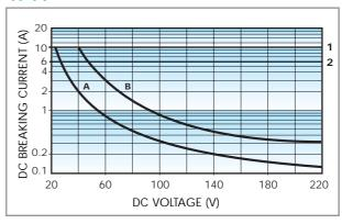
Breaking capacity for DC1 load.
