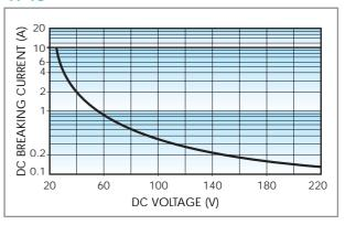
Breaking capacity in DC1 load.
