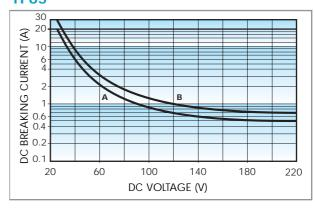
Breaking capacity for DC1 load. Load applied to 1 contact
