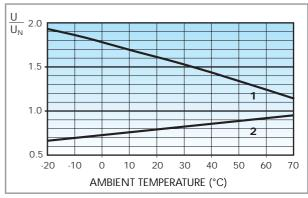
Operating range (DC type) vs ambient temperature.
