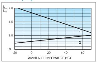
Operating range (DC type) vs ambient temperature.
