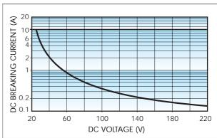
Breaking capacity in DC1 load.
