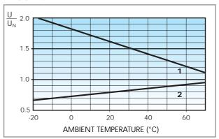
Operating range (DC type) vs ambient temperature.
