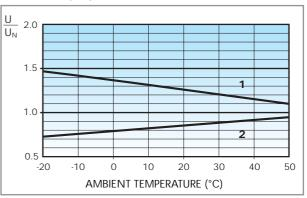
Operating range (DC type) vs ambient temperature.
