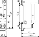
Clamp terminal socket: panel or 35 mm rail (EN 50022) mount
