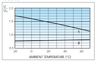
Operating range (AC type) vs ambient temperature.
