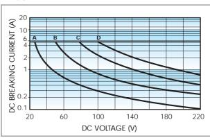
Breaking capacity for DC1 load.
