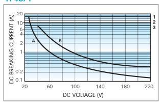
Breaking capacity for DC1 load.
