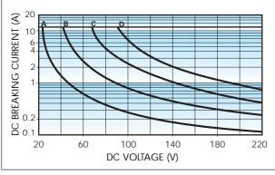
Breaking capacity for DC1 load.
