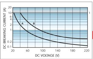
Breaking capacity for DC1 load.
