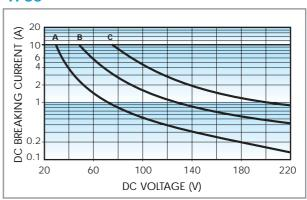
Breaking capacity for DC1 load.
