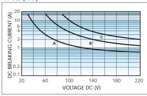
Breaking capacity for DC1 load.
