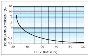
Breaking capacity in DC1 load.
