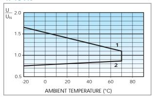
Operating range (AC version) vs ambient temperature.
