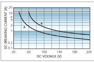
Breaking capacity for DC1 load.
