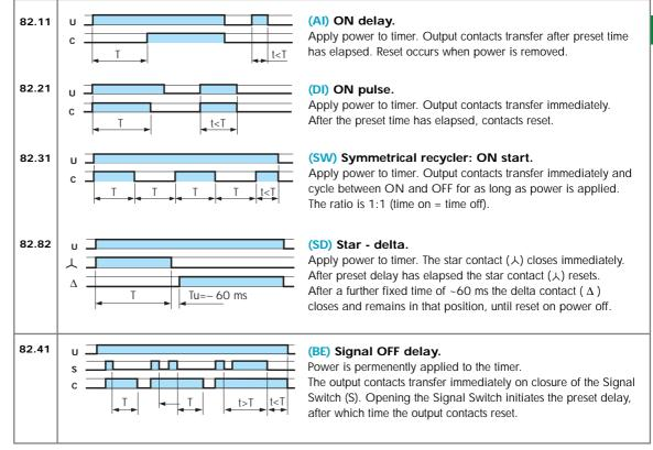
\* A voltage other than the supply voltage can be applied to the command START (B1). Example: A1 - A2 = 230 V AC/B1 - A2 = 24 V AC - Plug-in timer relay
