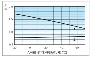
Operating range (AC type) vs ambient temperature.
