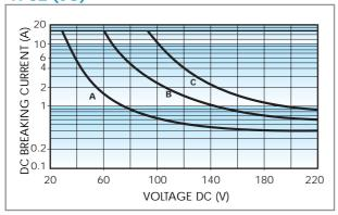
Breaking capacity for DC1 load.
