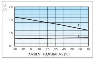
Operating range (AC type) vs ambient temperature.
