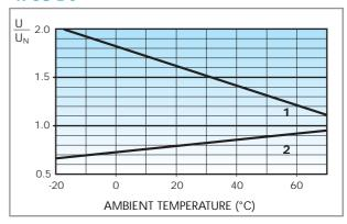
Operating range (DC type) vs ambient temperature.
