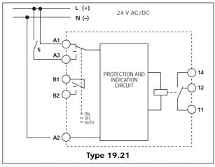
The max switching voltage between  $B_{\rm 1}$  and  $B_{\rm 2}$  terminal is 24 V AC/DC (300mA).
