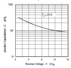
Fig. 3 Typical Junction CapacitanceVs. Reverse Voltage
