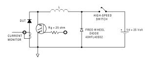
Fig. 8 Unclamped Inductive Test Circuit
