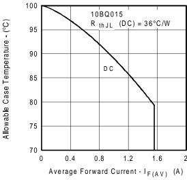
Average Forward Current - I<sub>F(AV)</sub> (Fig. 5 Max. Allowable Case Temperature Vs. Average Forward Current
