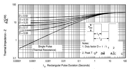
Fig. 4 Max. Thermal Impedance  $Z_{thJL}$  Characteristics
