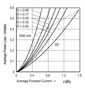
Fig. 6 Forward Power Loss Characteristics
