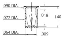
0479-0-XX-XX-34-XX-10-0 Solder mount in Ø.077±.003 PTH. #34 Contact for Ø.032-.046 pins. Also available on 16mm wide carrier tape: 2,000 parts per 13" reel.
