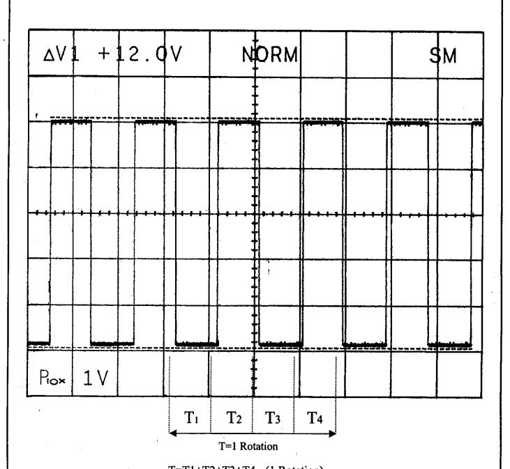
T=T1+T2+T3+T4 = (1 Rotation) $T1=T2=T3=T4= \frac{60}{4 \text{ (rpm)}}$
