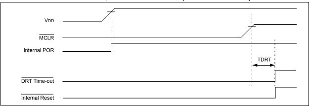
FIGURE 8-9: TIME-OUT SEQUENCE ON POWER-UP (MCLR TIED TO VDD): FAST VDD RISE TIME
