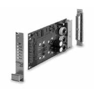
ADS\_E 50/5 4-Q-DC Servoamplifier Powerful PWM servoamplifier for permanent magnet activated DC motors from 10 to approx. 250 watts output power. Available as Standard Version in Eurocard format.
