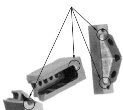
This Punch and Die are new and undamaged.
