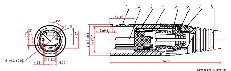
The pin plating silver, thickness 0.5μm (SOLDER).
