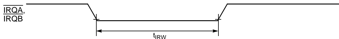
Figure 3-13 External Interrupt Timing (Negative-Edge-Sensitive)
