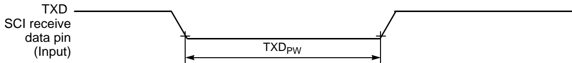
Figure 3-26 TXD Pulse Width
