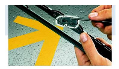
An adapter connects the blade assembly to the windshield wiper arm.
