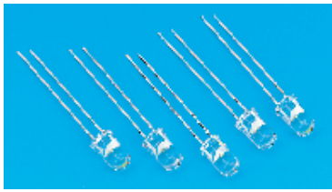
Dia = 5.0, L = 8.71, Leads = 22.89 0.5sq Lead Pitch = 2.54 Cathode identified by flat on body and shorter lead
