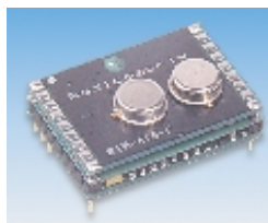
H = 23, W = 34, D = 12 (with pins) pins spacing 2.54 recommended PCB hole dia. 1.2
