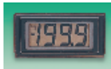
3 1/2 Digit (DPM125) SIL pins = 4 0.5 dia on 2.54 pitch
