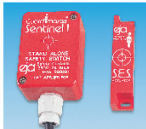
Switch H = 69, W = 50, D = 36 2 Mounting holes M4 Diagonally opposite 38 57 Actuator H = 82, W = 18 2 Mounting Slots M4 at 73 centres
