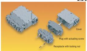
A range of polarised multipole connectors for cable to panel and cable to cable applications. The connector bodies are manufactured in **UL** approved polycarbonate. The plug and receptacle bodies can be loaded with solder, mini-wrap or crimp contacts as the application requires (all contacts fitting both the plug and the receptacle). The actuating screw eases mating and unmating of connectors, and secures mated connectors
