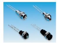
Bezel = 4 7 dia (Prominent), 3 7 dia (Recessed), Total L behind bezel = 11.5 (Prominent) 13.0 (Recessed), Mounting hole dia. = 6, Shorter lead Cathode
