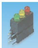
Viewed from front, pins downward, anode is right hand pin
