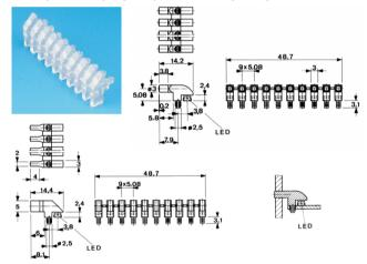
90° light pipe arrays for use with SMD LEDs. The 20 way units are a dual tier format and the 10 way units are single tier. The 20 way dual tier is available in  $3mm \oslash$  round section while the 10 way single tier modules are available in  $3mm \oslash$  and  $2mm \times 5mm$  rectangular. PCB mounted by 10 fluted pins. Temperature range = -40°C to +85°C OPT703b
