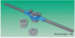
A kit comprising a die stock with screw in handles, two dies M20x1.5mm and M25x1.5mm with two centring guides
