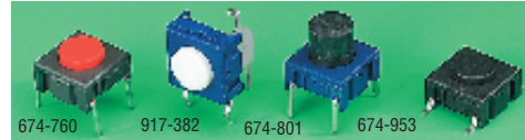
674-760 917-382 674-801 674-953 Body W = 10.1, D = 10.1, H (standard type) = 6.4, Button dia. = 6.5 PCB layout = 4 0.9∅ holes, rectangular formation, centres 10.16 7.62
