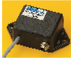
H = 20.3, W = 38 (body), 60 (overall), D = 32, Fixing centres = 50.8 (Dia. = 4.7), Cable L = 300 Connections: Brown = 5V, Green = 0V, White = Output
