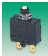
H = 32, W = 14, D = 27 Panel cut-out = 9.5 dia Tabs = 6.3 x 0.8
