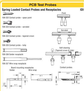
A range of professional spring loaded contact probes giving a full travel of 0.25" (6.35mm) designed to mate with either solder or wire-wrap receptacles. The probes are available with either a point, serrated or self cleaning tapered crown and tulip head styles and will suit most major manufacturers high speed vacuum ATE equipment.
