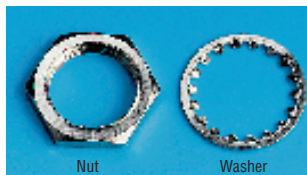
Nut 1/2" 28 UNEF 14 (14%) A/F 16 A/C Washer 17mm O/D 1.0mm Thick
