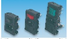
Cut-out 'A' Switched or fused/voltage selector or twin fused 151-746, 150-030, 150-032 Panel cut-out H = 48.4 W = 34.4, Thickness = 1.5 to 3 Depth behind panel = 38
