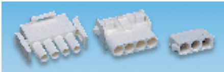
Plug housing Mates with receptacle or PCB header Cable or panel Mounting receptacle Panel thickness = 0.76-2.29 PCB header PCB hole dia = 1.8 Pitch = 6.35
